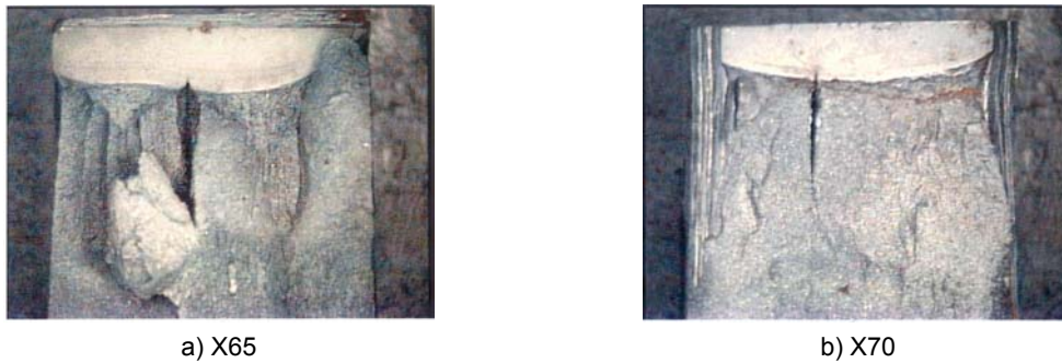
Figure 5: Specimen crack surface after CTOD test.
