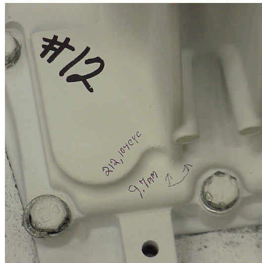
Figure 2B - Typical detectable crack. The maximum load on this sample was 2000 kN observed after 420,000 reversals
